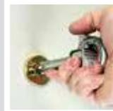
**2** Depress the safety catch then locate eyebolt into center of socket. Push the eyebolt with palm of hand until locking mechanism clicks.
