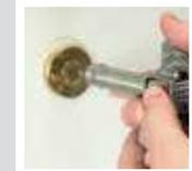
**4** When work is done, remove the lanyard from the eyebolt. With two hands, depress safety catch then trigger to remove the eyebolt from the socket.
